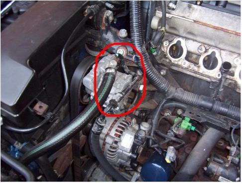
8, what i had to do was take the bracket off and undo the main bolt and rotate the pipe and then bend the bottom part slightly and the it cleared fine
