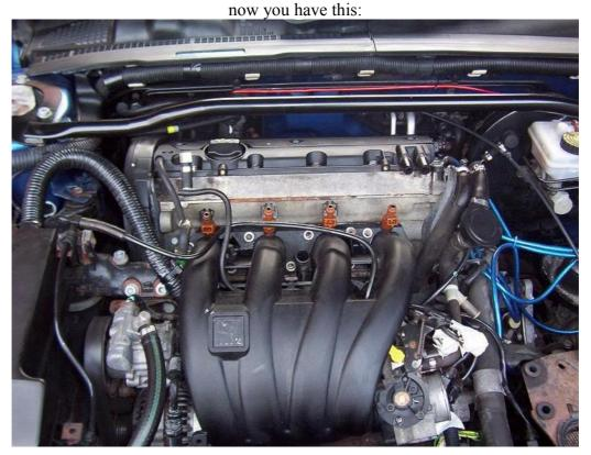
and then give the injectors a wiggle and a pull and they'll come out 7,right now its on to removing the manifold which is just a case of undoing some allen key bolts and some 13mm bolt aswell as a 10mm bolt near the dip stick one the are undone give the manifold a wiggle and it will come away now we have this:
