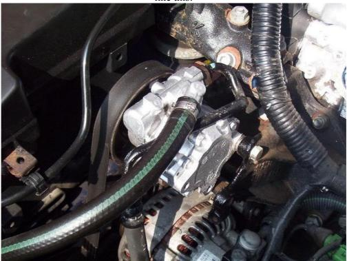
9, now we have to get the manifold ready to go on and start with the sensors, the sensors i swapped over from the original manifold where the map sensor, stepper motor and the air intake temp sensor and the are 2 wires that need extending and the first is the map sensor which needs extending 18" and the next is the throttle body heater plug (yellow one) by 12"
